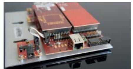
beroNet VoIP Gateways can be equipped with up to two modules which makes them very flexible and highly adaptable to a divers range of client requirements.
