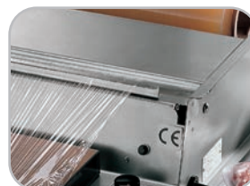
Particolare filo caldo (1) Heated cutting tread (1)
